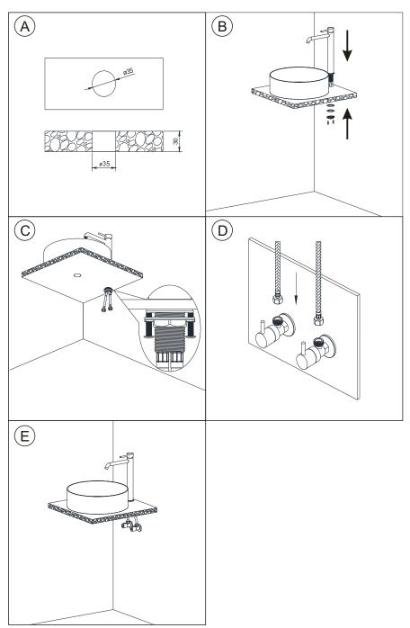
Tapware is to be installed by a Licensed Plumber in accordance with Recommended working water pressure 300-500 kpa. Maximum water temperature is 65 deg.c
